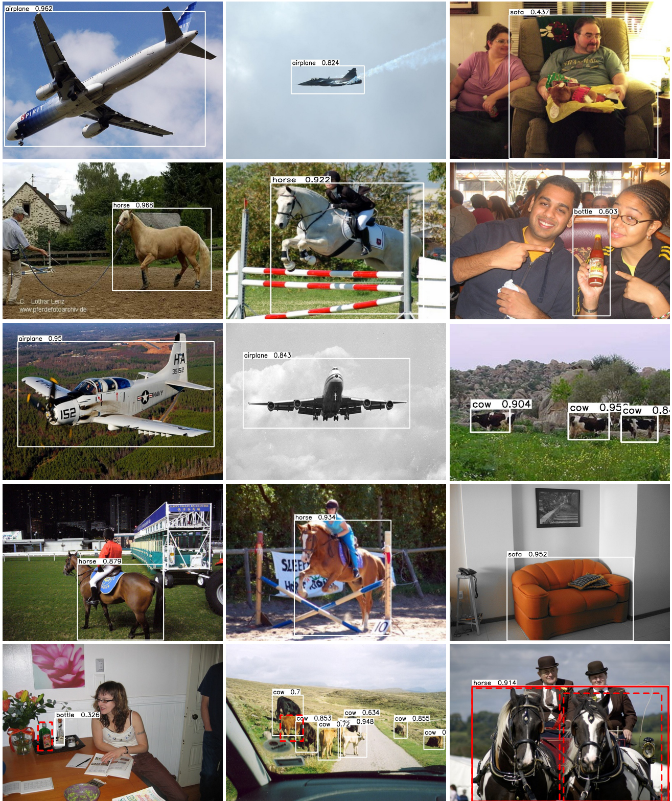
Figure 11. Visualization of multi-scale Meta-DETR’s 10-shot object detection results on Pascal VOC category split 2. Novel categories include airplane, bottle, cow, horse, and sofa. For simplicity, only results of novel categories are illustrated. White boxes indicate correct detections. Red solid boxes indicate false positives. Red dashed boxes indicate false negatives.
