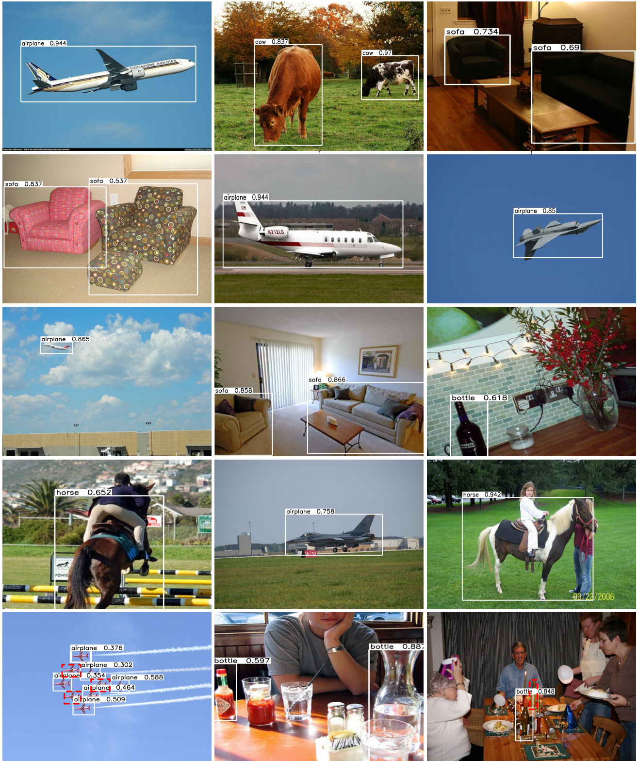
Figure 10. Visualization of multi-scale Meta-DETR’s 10-shot object detection results on Pascal VOC category split 2. Novel categories include airplane, bottle, cow, horse, and sofa. For simplicity, only results of novel categories are illustrated. White boxes indicate correct detections. Red solid boxes indicate false positives. Red dashed boxes indicate false negatives.
